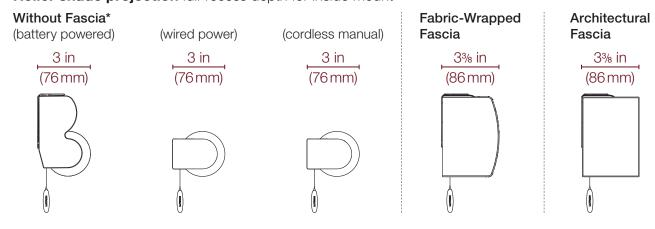
\* Without fascia, the projection varies with the size of the fabric roll-up (fabric panel height). The dimension shown is based on the largest available fabric panel height; the **maximum** projection.
