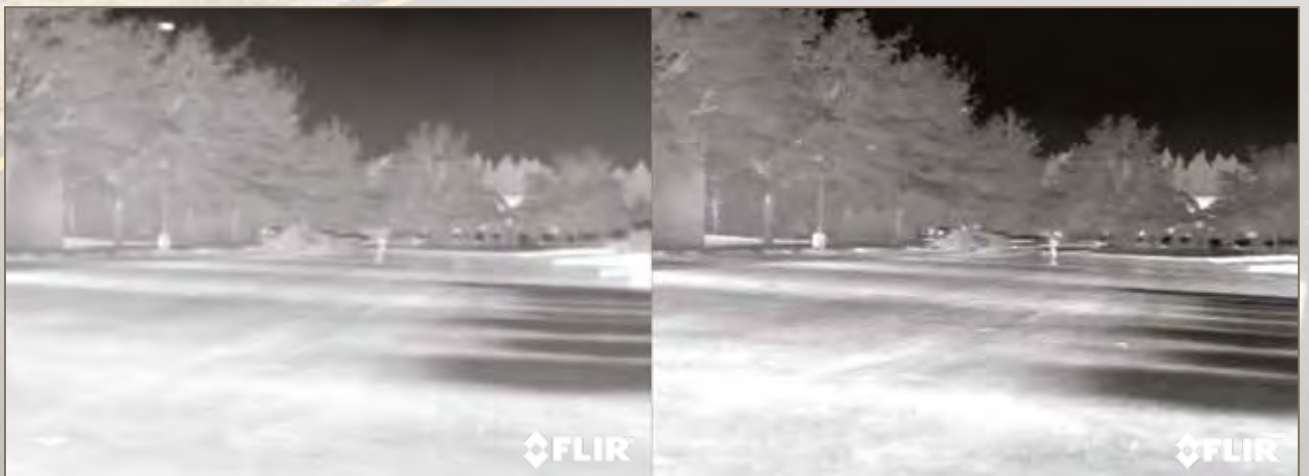
The 320x240 pixel resolution image on the left shows less image detail than the 640x480 pixel resolution image on the right.
