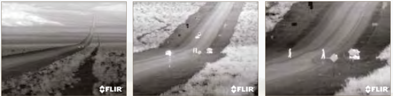
How far you can see depends on many factors including the size of the object you're looking at, and the focal length of the lens you're using. These three images all show people and cars from 2 km away, but they look very different because they use different lenses.
