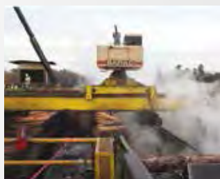
Operators cannot see through the steam cloud caused by condensation in cooler air temperatures.
