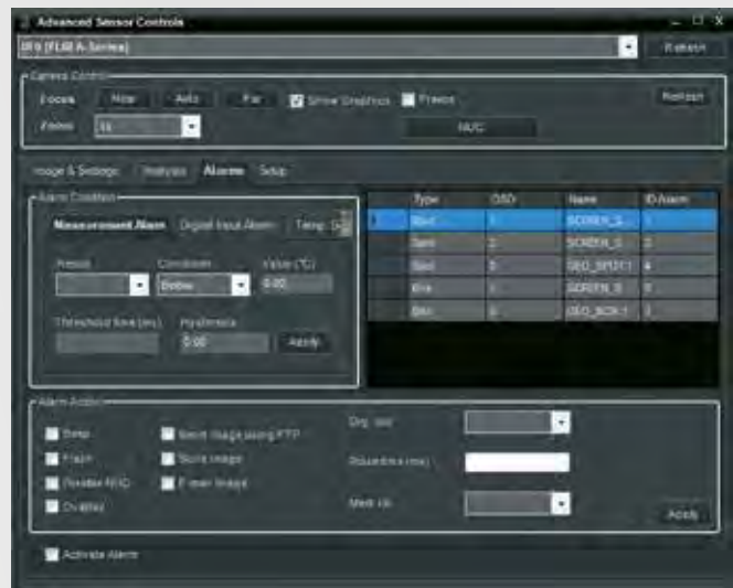
FLIR Sensors Manager allows for easy setting of alarm conditions and alarm actions
