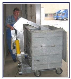
The compactor can be used in- and outside. Open the lid of the container and push the container onto the plattform of the compactor. The compaction plate must be lifted. There is enough space for filling in. When the container is full, the compaction plate manually operated with two hands compacts inside the bin. It is absolutely
