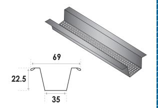
The use of Furring system is to give the surface a smooth look in the ceiling system and it helps to cover the installed air conditioning ducts and other visible wiring. It is also used on walls where many / any objects are to be hidden. The Furring system is the combination of Furring Channel, Wall Angle and Main Channel to form a grid for suspended ceiling to be covered with the gypsum board.
