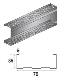
Any size of Stud range from Stud 40mm up to Stud 198mm can be produced. Flange height can be made up to 60mm.
