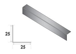
The regular size of this profile is 25x25mm, but we can produce in various sizes, lengths and thicknesses. The fixing of Wall Angle makes a firm platform for Ceiling Furring Systems. It is also being used to protect the edges and corner of installed gypsum board.
