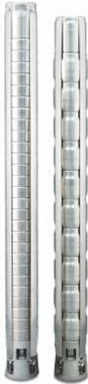
**Description :** C.R.I. 6" Stainless Steel Submersible pumps are made of corrosion resistance Stainless Steel with inbuilt check valve. All vital components are made of high quality 304 / 316 grade Stainless Steel and the shaft is of SS 304 / 329 / 431. The optimal design of impellers and diffusers enables the best possible hydraulic efficiency.
