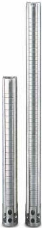
**Description :** C.R.I. 4" Stainless Steel Submersible pumps are made of corrosion resistance Stainless Steel with inbuilt check valve. All vital components are made of high quality 304 / 316 grade Stainless Steel and the shaft is of SS 304 / 329 / 431. The optimal design of impellers and diffusers enables the best possible hydraulic efficiency.
