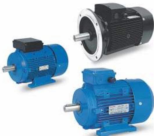
**Description :** C.R.I. A.C. Induction motors are high efficient suitable for continuous duty operations. Motor stator is made of low watt loss steel laminations assembled under pressure and rigidly locked in the stator frame. Dynamically balanced rotor ensures vibration free and noise free operations. The varnish impregnated windings are made of high-grade enameled copper wire.
