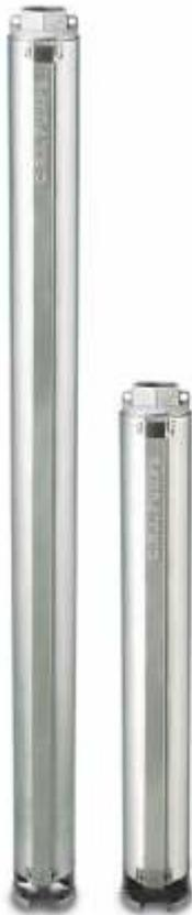
**Description :** C.R.I. 4" Silver line series Submersible pumps are built with thermoplastic impellers, diffusers and inbuilt check valve. All vital components of these pumps are made of corrosive resistance thermoplastic and the shaft is of AISI 304 / 431. Pumps are multistage centrifugal type. The optimal design of impellers and diffusers enables the best possible hydraulic efficiency.
