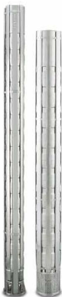
**Description :** C.R.I. 8" & 10" Stainless Steel Submersible pumps are made of corrosion resistance Stainless Steel with inbuilt check valve. All vital components are made of high quality 304 / 316 grade Stainless Steel and the shaft is of SS 304 / 329 / 431. The optimal design of impellers and diffusers enables the best possible hydraulic efficiency.
