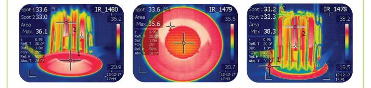
The primary influencing factor prevailing negatively upon LED life and efficiency is high temperature. The NT10 has been designed to operate with a junction temperature of less than 60°C and the excellent thermal efficiency of its heat-sink design extracts and dissipates this heat in a highly efficient manner.
