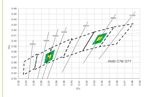
LED Evolution follows the ANSI recommendation that lamp manufacturers select LEDs from within a 4 step ellipse of any correlated colour temperature (CCT) target point.
