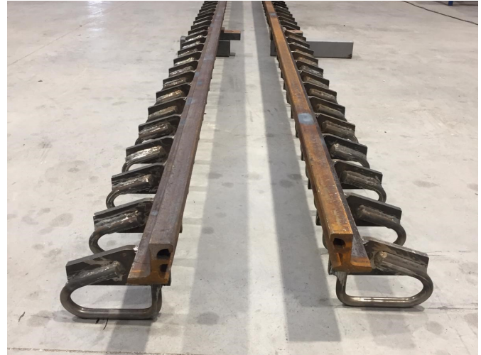
Fabrication of AR-EX HS—Before Painting
