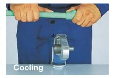
6. It is recommended to keep the connection fixed for the next 10 - 20 seconds, allowing the weld to cool down partially and achieve the initial strength. It is now possible to make other connections of the system. Full load of the weld is allowed only when the connection has cooled down completely.
