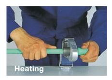
4. Simultaneously insert the pipe end and slide the fitting over corresponding heating tips of the welder (heated up to 260 - 280° C earlier) Keep the required heating time - see heating time values for different system dimensions.
