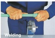
5. After heating, remove both elements from heating tips and push the pipe into the fitting flange up to the depth marked earlier. The welding time depends on the outer diameter of the pipe. Good welds should have a double, uniform fin of material pushed out to the surface, along the circumference connected elements.
